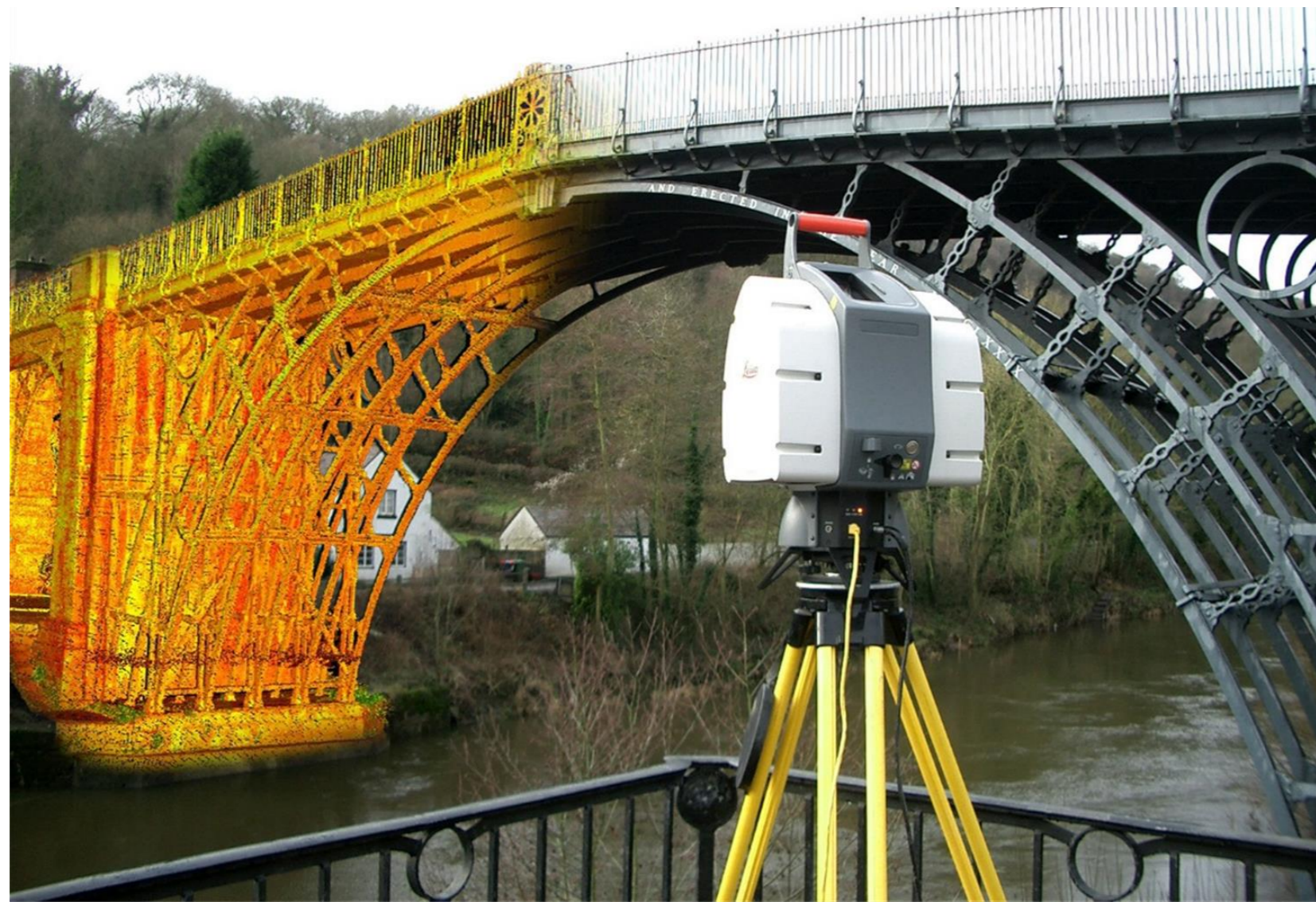
Laser Scanning to Revit
