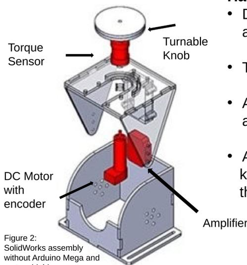
Figure 2: SolidWorks assembly without Arduino Mega and motor shield
