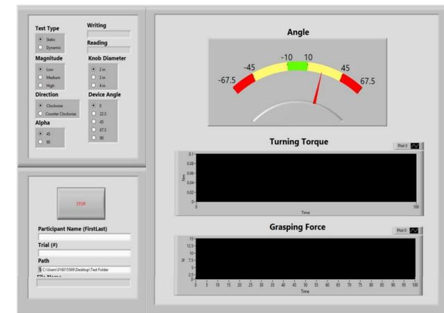
Figure 6: GUI designed in LabVIEW
