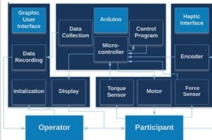
Figure 5: System design layout
