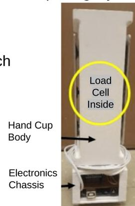
Figure 1: Grip-Load Device
