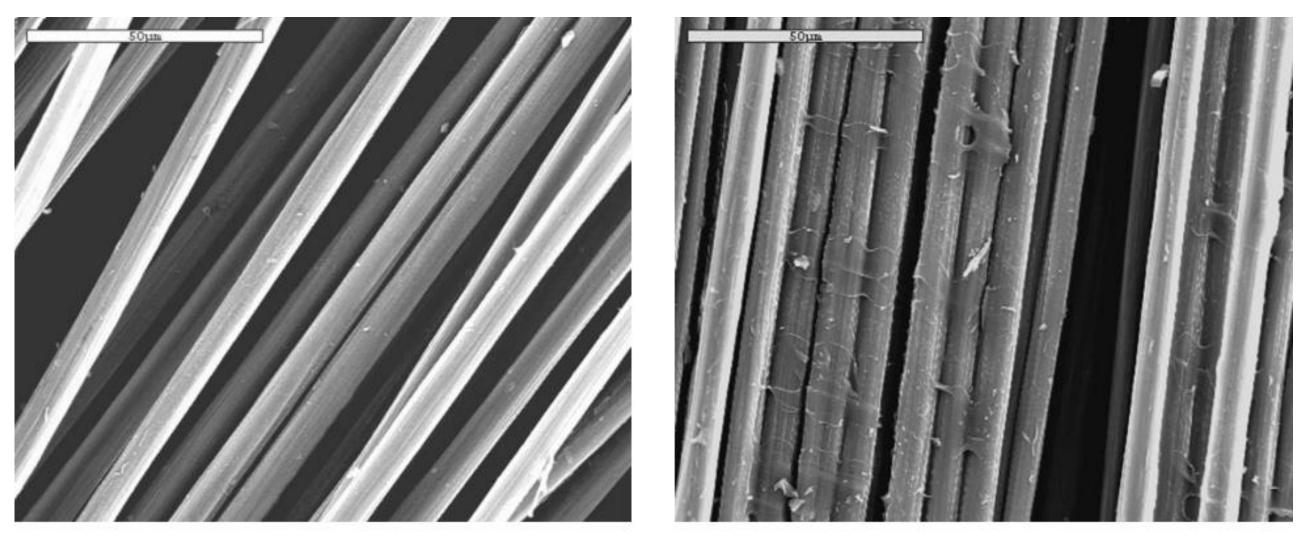
(b) Recycled fibres with char residue. (a) Clean recycled fibres. Fig 3. A comparison between the recycled fibers with (a) and without (b) an
