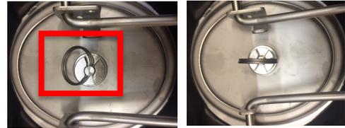
**NOTE: even if you don't need to fill sheath tank, you still need to close the pressure loop!**
