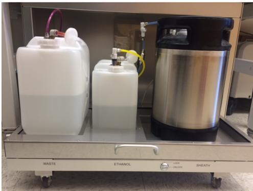
**Please** be gentle when removing and replacing tanks. The cart contains sophisticated balances to measure volume in the tanks. **Do not drop the tank back onto the cart when full!**
