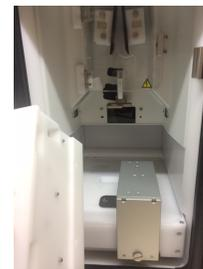
Plate holder – can be pre-chilled in freezer. Must put in plate holder attachment to hold plate. Can sort into PCR plate or regular 96-well plate
