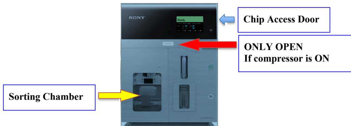
• **LASER SAFETY.** This device is considered a Class I laser device or one that does not produce injurious laser emissions accessible to the operator under normal operating conditions. Within the enclosed system are higher power Class 3B potentially injurious lasers. The user is protected from harmful laser emissions by the equipment housing and the sorting chamber door interlock switch. NEVER attempt to remove equipment housing components or disable the sorting chamber door interlock.
