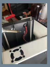
As I was starting to test the dimensions, I discovered a wire that's essential to the printing process ripped but luckily a quick solder fixed it.
