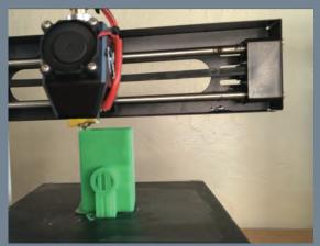
After I finished modeling on Solidworks, I saved the file as an STL file type, uploaded the file into the 3D printing software called Cura, saved the file as a gcode, uploaded the gcode into a micro SD card, inserted the card into the printer, and printed the parts.
