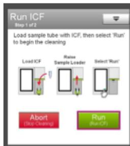
5. When the ICF cycle is complete, the system prompts you for a tube of DI water. Load a full tube of DI water on the unit and select **Continue**.
