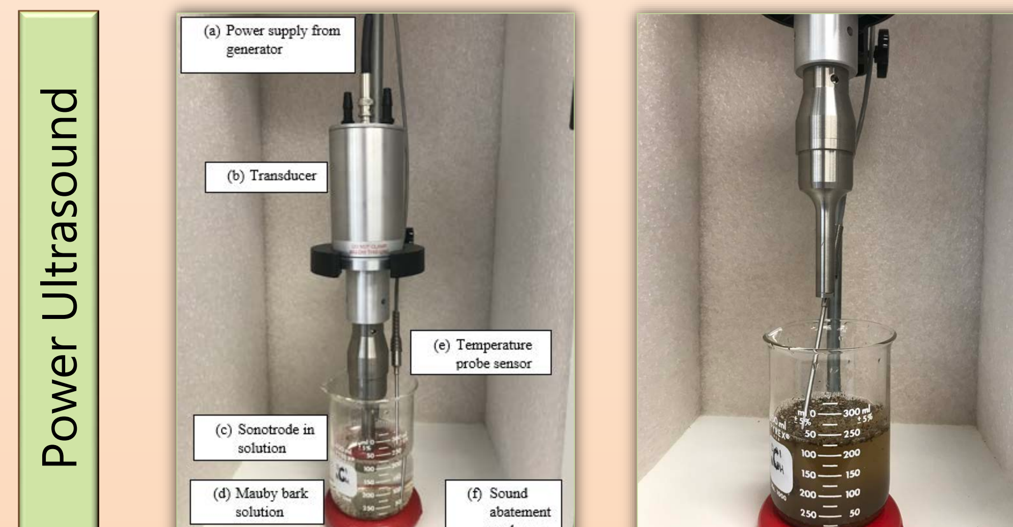
Figures 5A and B. (A) PU assembly begins with (a) the power supply cord from the generator, which is attached to (b) the transducer for the energy to be transferred into ultrasonic waves via (c) the sonotrode inserted directly into (d) the Mauby bark powder in ddH 2 O. To measure temperature, (e) the temperature probe sensor is also inserted in the solution. All of which is enclosed in (f) the sound abatement enclosure to minimize the noise resulting from ultrasonic processing; and (B) processing of powdered Mauby bark. 7
