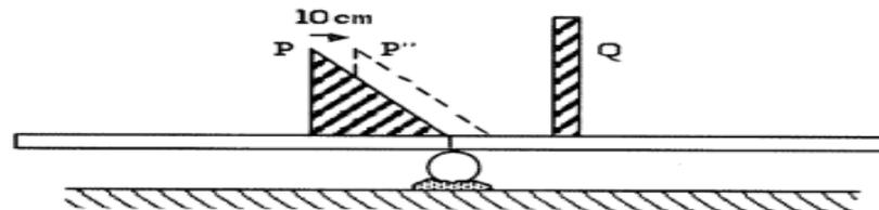
To keep the system balanced, should object Q be moved a distance *greater than*, *less than*, or *equal to* 10 cm? Explain.
