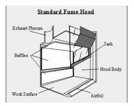
Figure 1. Basic features of a chemical fume hood.
