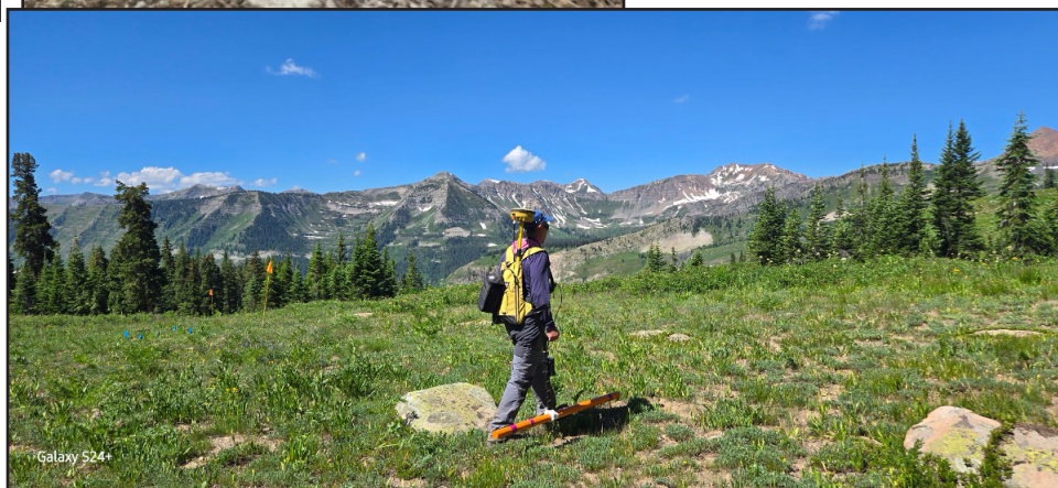
Matt Becker collecting Frequency-Domain Electromagnetic (FDEM) data in Crested Butte, Colorado
