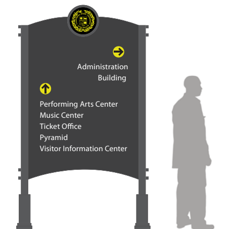
ROADWAY DIRECTIONAL SIGN 2 Fabricated, aluminum sign panel with applied vinyl and/or screen printed graphics, and cast aluminum University Seal plaque, supported by round aluminum posts.
