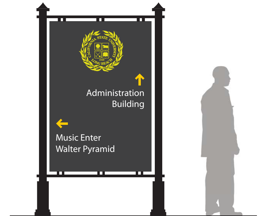
ROADWAY DIRECTIONAL SIGN Fabricated, aluminum sign panel with applied vinyl and/or screen printed graphics, and cast aluminum University Seal plaque, supported by round aluminum posts.
