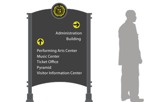
ROADWAY DIRECTIONAL SIGN SMALL Fabricated, aluminum sign panel with applied vinyl and/or screen printed graphics, supported by round aluminum posts.
