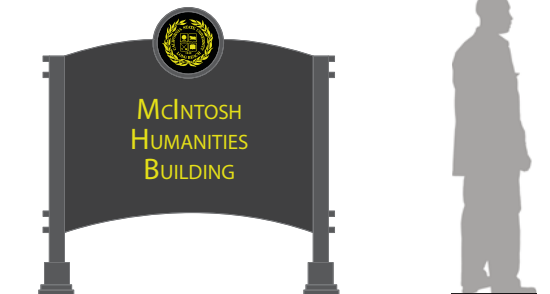
PRIMARY BUILDING ID SIGN Fabricated aluminum sign panel with precision cut, solid bronze letters, with clear protective finish. Letter faces to be brushed and returns to be bead blasted, supported by round aluminum posts.
