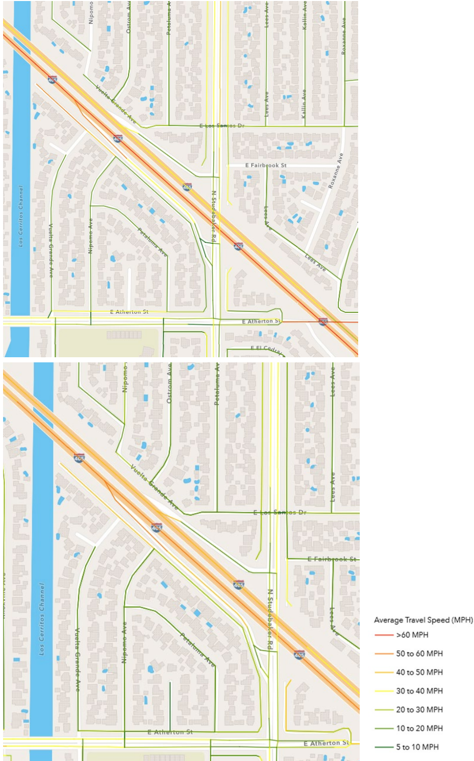
Figure 3. Wejo Average Speed by Segment AM Peak (Top) & PM Peak (Bottom) at Study Location 3: I-405 at Studebaker Road
