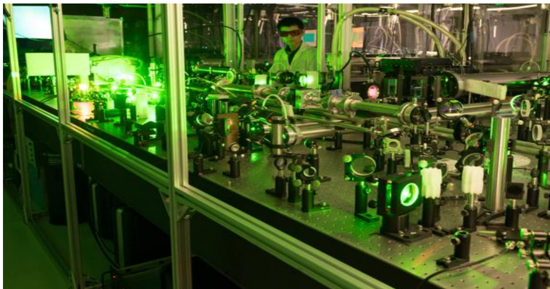
Figure 1. Ultrahigh power laser. The green laser beams energize Ti:Sapphire crystals that amplify light at 800 nm wavelength.
