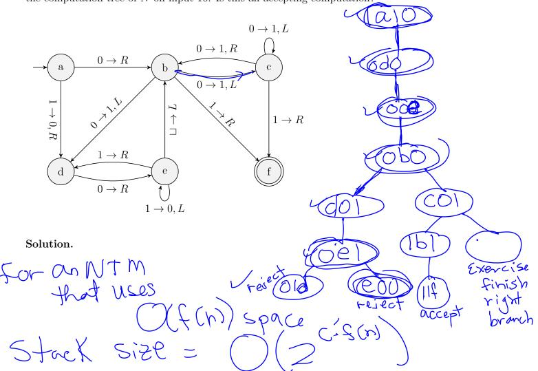
**Example 4.** Provide a state diagram for a nondeterministic Turing machine M that starts with a blank input tape and proceeds to generate eight different configurations, with each configuration having the form  $wq_3 \sqcup$ , where  $w \in \{0,1\}^3$  and no two configurations have the same binary word.
