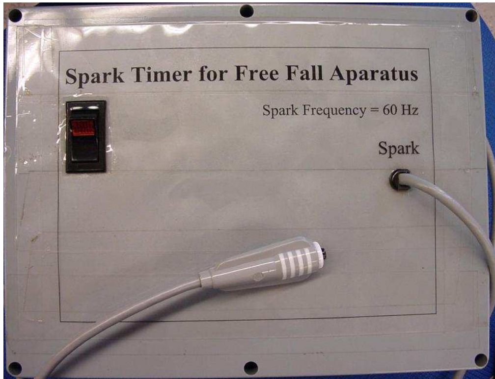
Figure 4: This is the box I designed and built. A 12V ignition coil inside the box produces the spark. Additional circuitry is included to make the apparatus spark every 1/60 th of a second.
