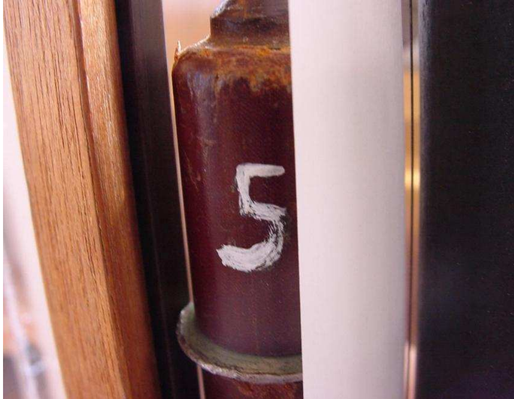
Figure 2: A spark jumps from the wire on the right, through the paper, to the metal ring on the falling bob. Then the spark jumps again from the metal ring to the metal rail on the left, completing the circuit.
