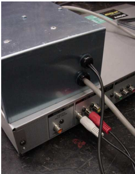
Figure 2: The left and right channels from the audio output of the DVD player are used as the input signals to the accessory device.
