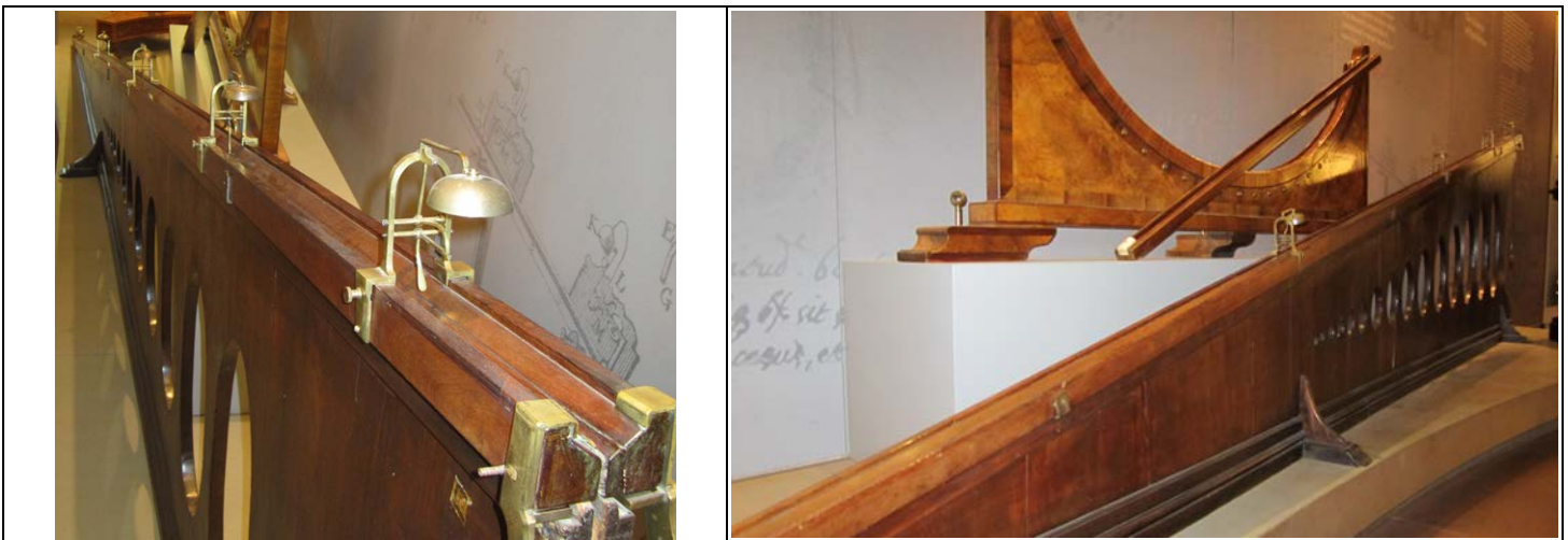
Pictures of the actual inclined plane apparatus used by Galileo to test the principle of universal gravitational acceleration and determine a value for g . Balls rolled down the tracks ringing bells to help with timing. The inclines could be changed in some cases to increase or decrease the vertical component force of g accelerating the balls. From: Arbor Scientific 116
