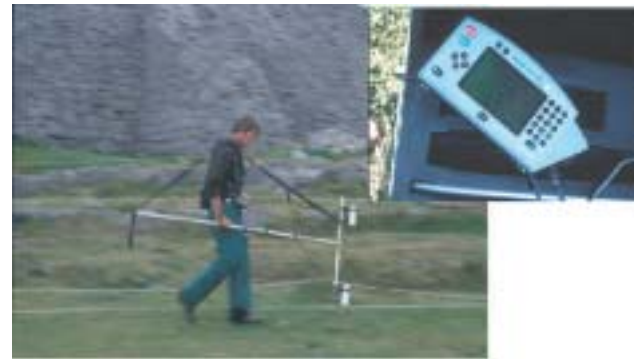
Figure 2 Gradiometer survey in progress. The insert shows the panel of the Geometrics 858 instrument and display.
