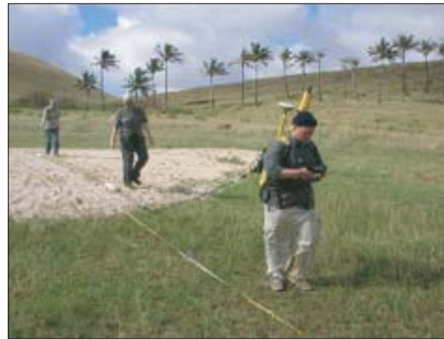
Figure 1 Students on Rapa Nui, Chile conducting a resistivity study of Anakena. The resistivity unit consists of a data collector and integrated GPS system.
