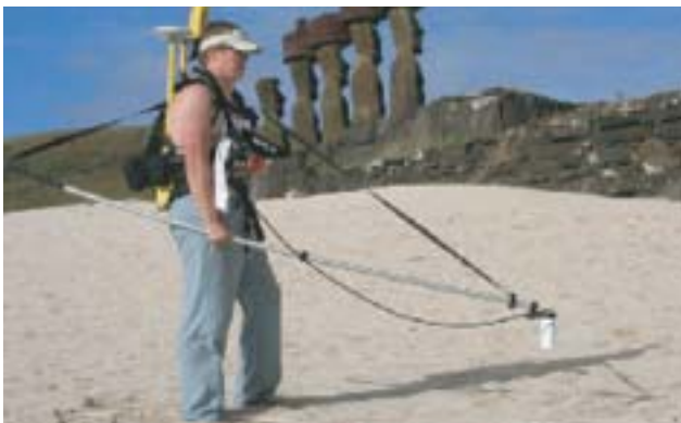
Figure 13 A CSULB student using the integrated real-time kinematic global positioning system and magnetometer. This integrated design allows one to simultaneously collect magnetic and spatial information.
