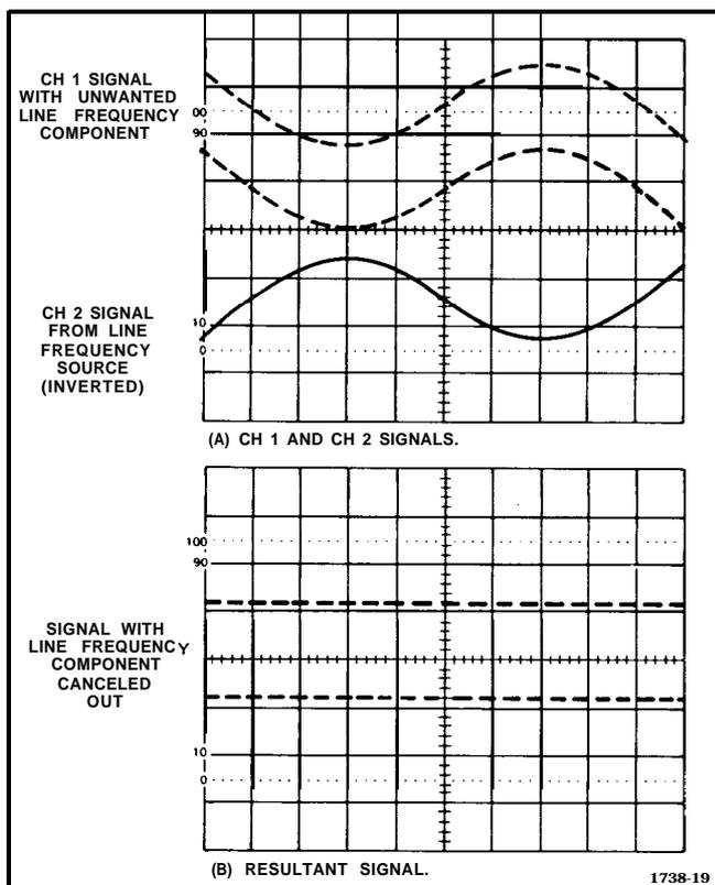
Figure 14. Common-mode rejection.
