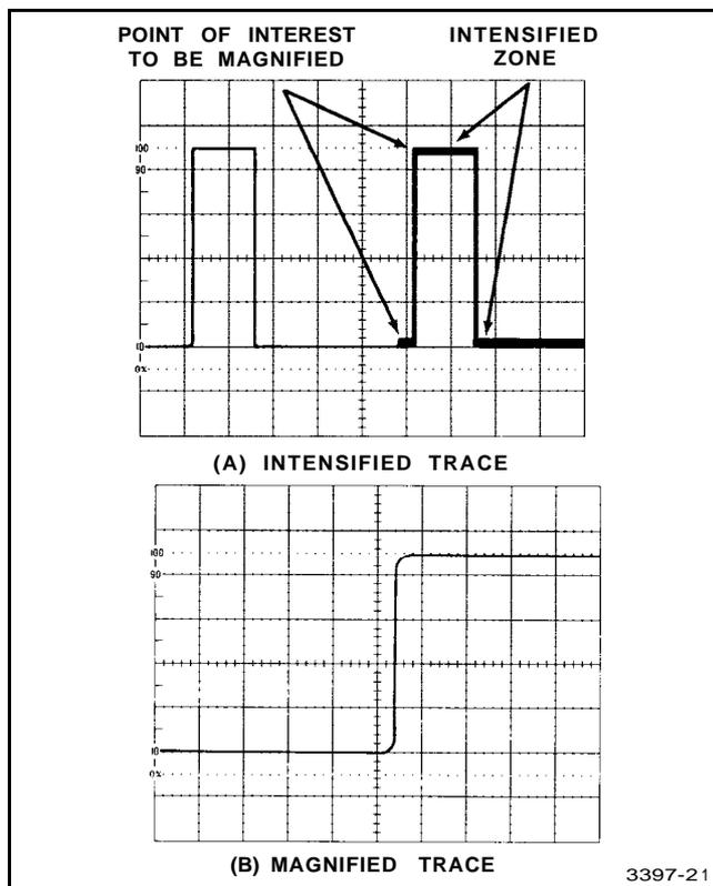
Figure 20. Delayed-sweep magnification.
