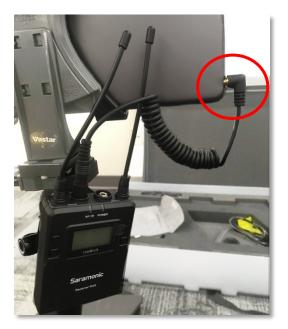
2. Attach the microphone to your lapel, and turn on the transmitter.
