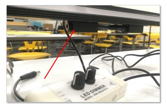
2. Connect the remaining light dimmer switch cable to the power supply adapter and plug into an outlet.
